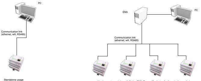
Used as system solution with Netico EMA (Energy Monitoring Appliance) – for monitoring large complex installations
