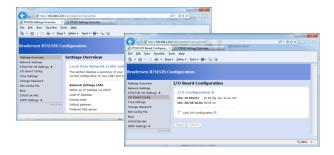
Basic configuration using Internet Browser connected to the integrated WebServer. Configuration include e.g. basic settings for network communication, I/O configuration and SNTP (time synchronization via Simple Network Management Protocol) etc.
